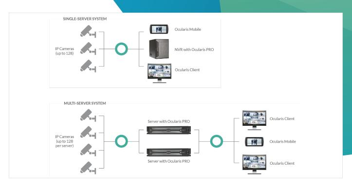
System diagram: In smaller systems, all Ocularis components may be installed on the same PC/server.
